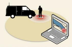
By collecting signal strength in several locations, the system can triangulate and map a phone's location.
