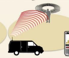
2. The stingray system, which mimics a cellphone tower, gets the target phone to connect to it.
